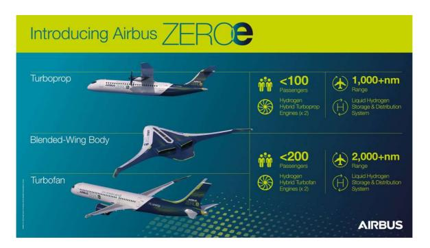
AIRBUS ZERO E - https://www.airbus.com/innovation/zero-emission/hydrogen/zeroe.html
